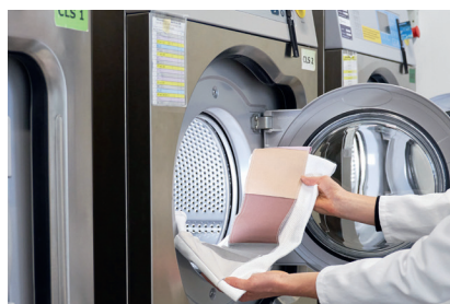
Abb. 2: Standard-Stain-Strip, gemäss ICE60456.
